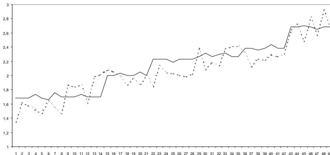
Fig. 4. Real values of cutting forces on the first tool of the set (continuous line) and their predictions (dot line) - RBF 3-6-3 network, test set of the experimental data
