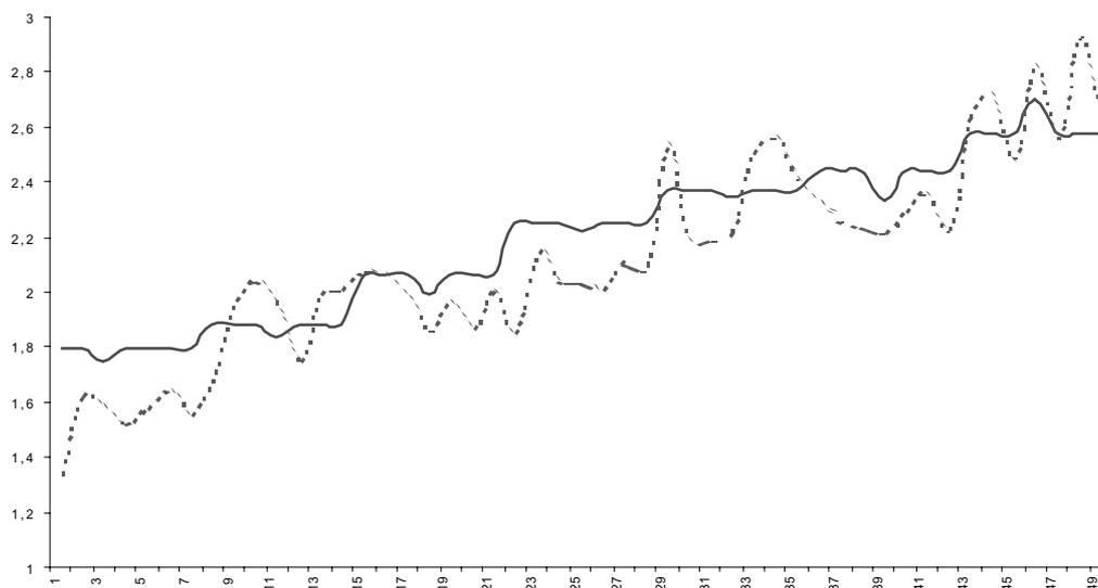
Fig. 2. Real values of cutting forces on the first tool of the set (continuous line) and their predictions (dot line) - GRNN 3-95-4-3 network, test set of the experimental data
