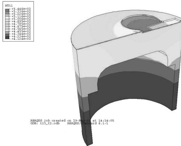
Fig. 4. Temperature distribution in the piston covered with TBC's at 12ms
