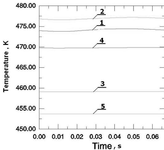
Fig. 3. Temperature variations throughout the cycle at the metal surface
