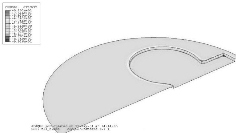
Fig. 7. Distribution of normal component of stress at bond coat/substrate interface at 15.5 ms
