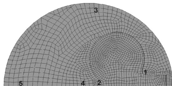
Fig. 1. Piston model, mesh and locations of points
