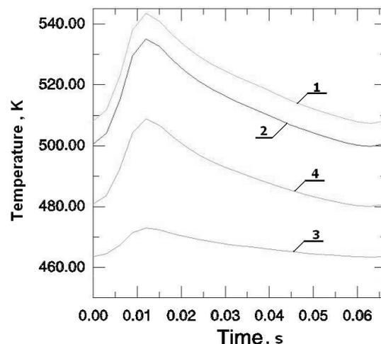
Fig. 2. Temperature variations throughout the cycle at the TBC's surface
