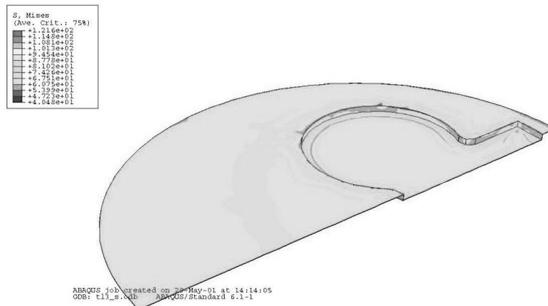
Fig. 6. Distribution of von Mises' stresses at the TBC's surface at 12ms
