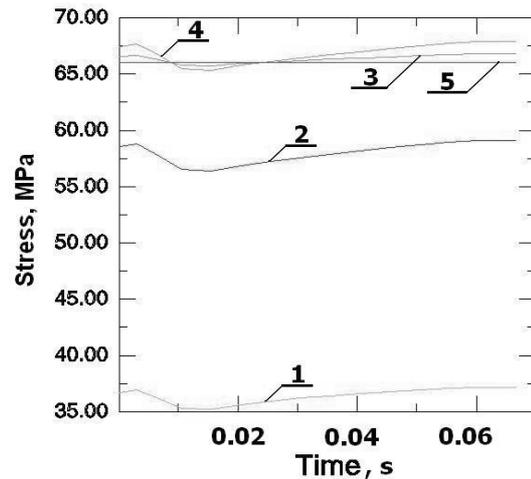
Fig. 5. Variation of von Mises' stresses in the cycle at the TBC's surface
