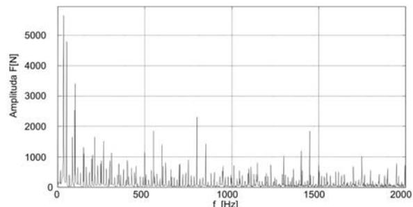
Fig. 3. Amplitude spectra of simulated response of bearings in a toothed gear with 2<sup>nd</sup> degree pitch error the pinion
