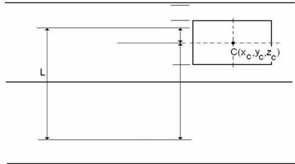
Fig. 4.1. The maximum (admissible) width  $L$  of the set  $\Omega$  between the mass centre of the car model and the roadside: Source: authors' own research
