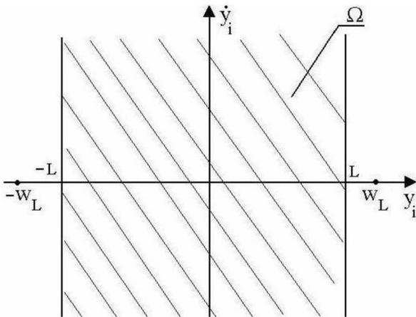
Fig. 3.1. Illustration of  $\Omega$  for the lateral translation of a railway car [3]
