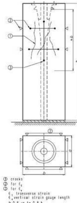
Fig. 4. Measuring set-up for load transfer test
