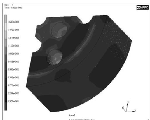
Fig. 17. Distribution of stresses in the anchoring block
