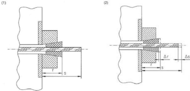
Fig. 1. Slides in the anchorage: a) anchorage before prestressing, b) anchorage after prestressing
