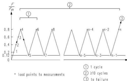
Fig. 3. Course of specimen load
