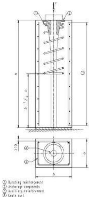
Fig. 2. Test specimen for load transfer test
