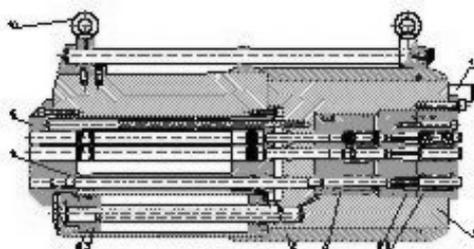
Fig. 7. Multi-cables press: 1 – major piston, 2 – cylinder, 3 – succor pistons, 4 – front block, 5 – front rosette, 6 – back rosette, 7 – disc of disanchor pistons, 8 – disc of inner jaws, 9 – pistons of the anchor external jaws (in the anchor block), 10 – respite, 11 – sensor of the protrusion of piston
