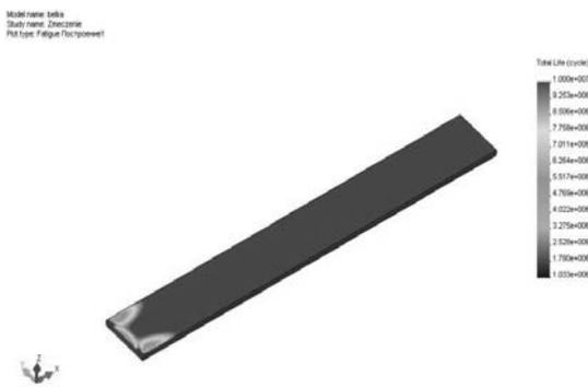
Fig. 3. Life cycle fatigue map of the laminate beam
