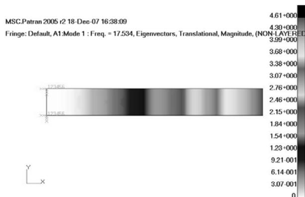
Fig. 2. Map of the normal mode of the laminate beam
