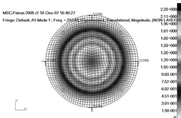
Fig. 1. Map of the normal mode of the laminate plate
