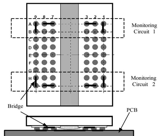
Fig. 2 Monitoring circuit with bridge
