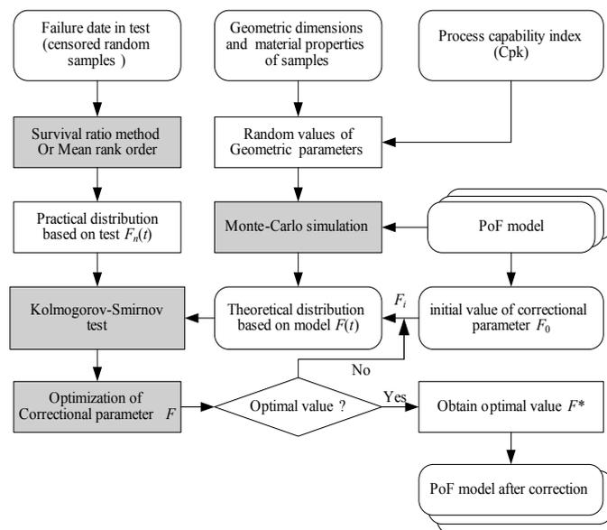
Fig. 1. The process of model modification method
