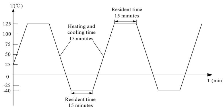
Fig.3 The typical temperature stress profile in the test
