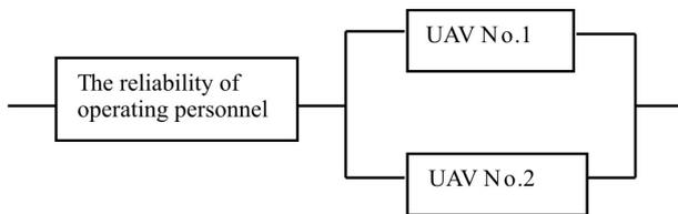
Fig. 3. The UAV total system mission reliability diagram
