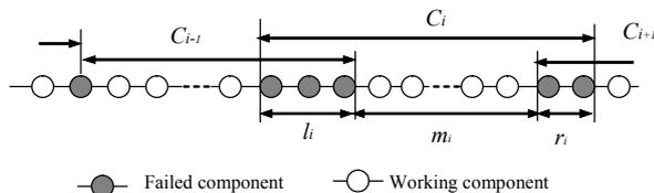
Fig. 1. Illustration of division of subsystems
