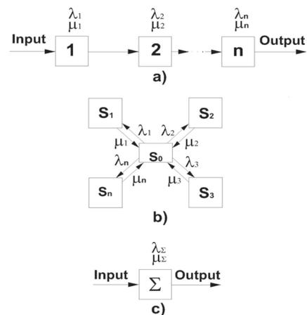
Fig.1. The conditions graph of the multirole CNC machine tool: a) system elements from 1 to n; b) elements conditions; c) machine as the sum of all elements
