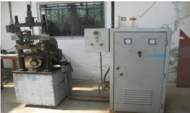
Fig. 2. The test bench for the fatigue testing of specimens
