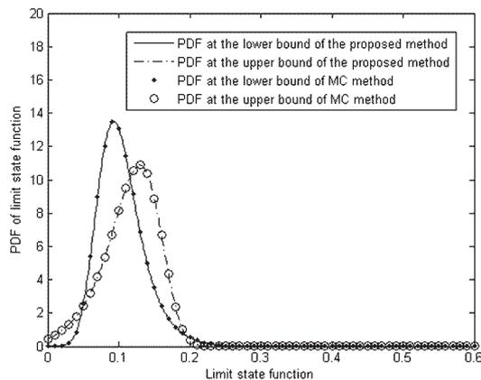
Fig. 4. PDF of the limit state function for clutch
