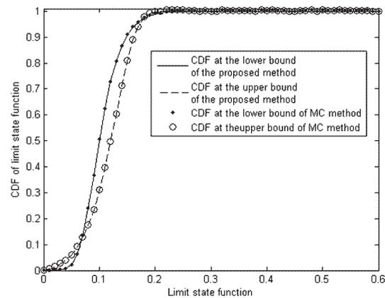
Fig. 5. CDF of the limit state function for clutch
