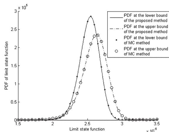
Fig. 2. PDF of the limit state function for disk edge design
