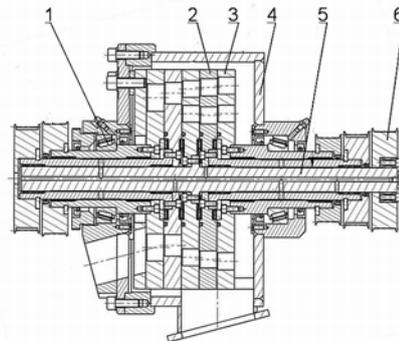
Fig. 3. The working unit of the five-disc, multi-hole RWT-5KZ grinder [4]: 1- bearing, 2- grinding disc, the so-called „preceding” disc, 3- grinding disc, the so-called “next” disc 4- body, 5- shaft, 6- pulley
