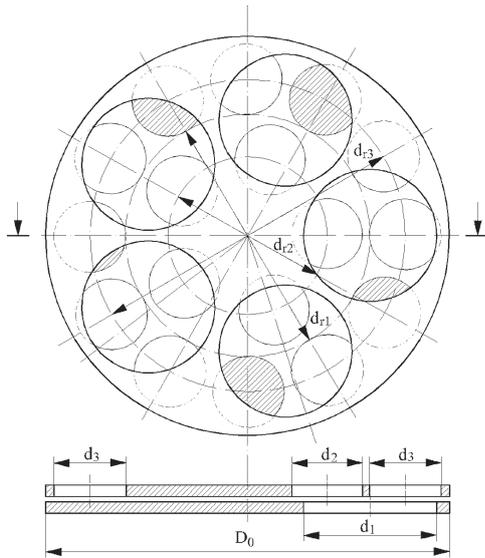
Fig. 1. Design features, cross-sectional area and effective grinding surface for two grinding working discs between cutting edges [5]:  $D_0$ —outer disc diameter;  $d_{r1}$ — diameter of working holes mounting in the preceding disc,  $d_{r2}$ — mounting diameter of working holes inner row in the next disc,  $d_{r3}$ — mounting diameter of working holes outer row in the next disc,  $d_1$ — diameter of working hole in the preceding disc,  $d_2, d_3$ — diameters of working holes in the next disc.
