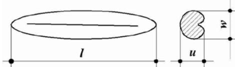
Fig. 2. Model of the geometric form of the basic grains:  $l, u, w$  – maximum dimensions of grain within three planes
