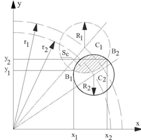
Fig. 6. Common area of two holes, grinding cross-section between the edges of neighbouring grinding holes:  $C_1, C_2$  - working holes centres,  $R_1, R_2$  - working holes radiuses,  $r_1, r_2$  - working holes positioning radiuses,  $x_1, x_2, y_1, y_2$  - coordinates for  $B_1$  and  $B_2$  quasi-cutting pair circles intersection points,  $S_C$  - quasi-cutting hole pair common area
