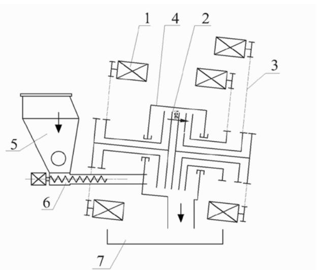
Fig. 4. Kinematical diagram of the multi-disc with inclined axis of working disc rotation for gravitational facilitation of feed movement: 1-electric motor, 2-grinding discs, 3-gears, 4-working space body, 5-container, 6-feeding screw, 7-finished product tank
