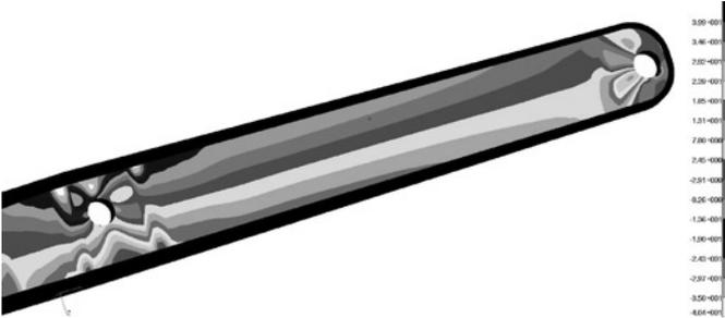
Fig. 16. Stresses in the bayonet part of spar
