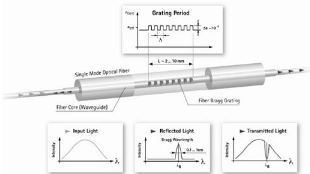
Fig. 22. Principle of Bragg gratings [HBM GmbH]
