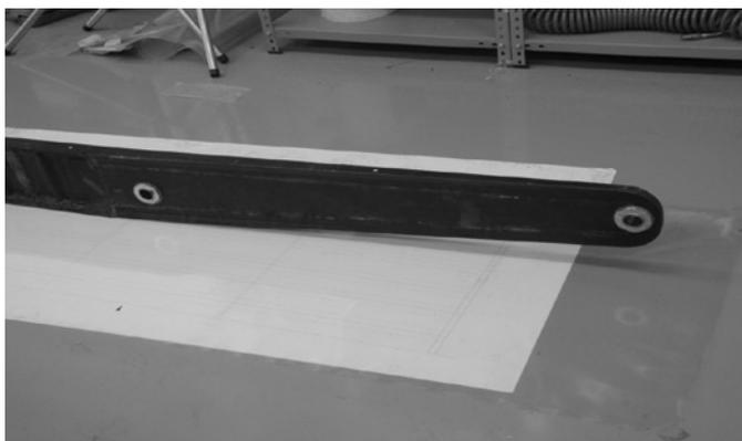
Fig. 8. Bayonet part of the tested spar
