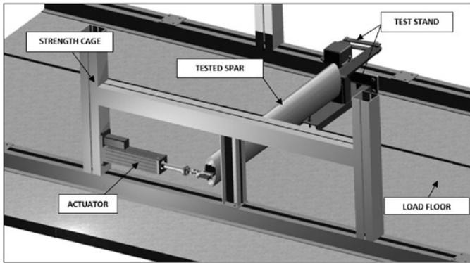
Fig. 2. CAD model of test stand
