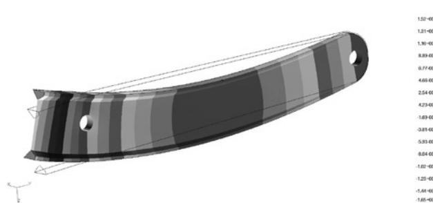
Fig. 14. Spar deflection. Result of FEM analysis. Load  $n=-3.7$
