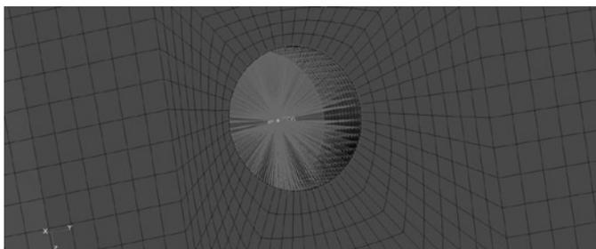
Fig. 10. Part of FE mesh and 1D elements simulating fittings
