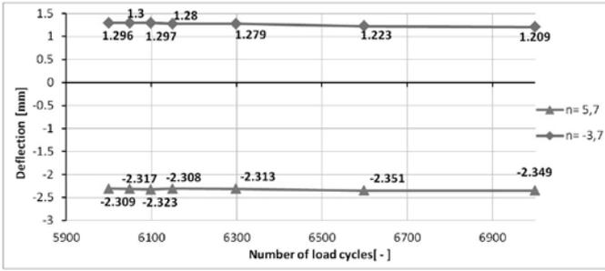
Fig. 15. Changes of deflection during the test
