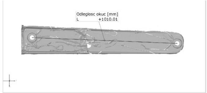
Fig. 19. Spar scan after 5,000 load cycles
