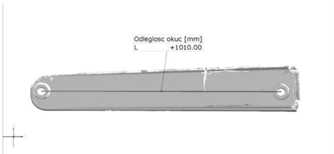
Fig. 18. Spar scan after 2,000 load cycles
