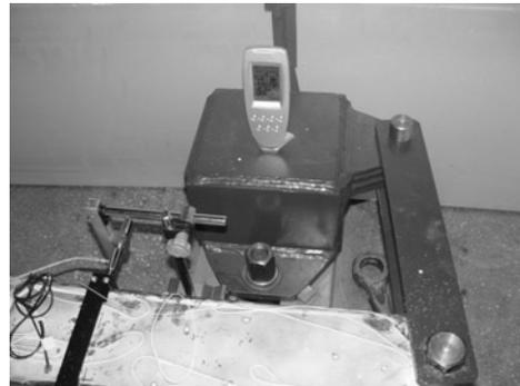
Fig. 11. Attachment of the inductive sensor
