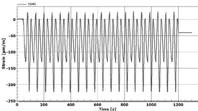
Fig. 23. Example of the strain history of strain gage number 1545 (around the front fitting) -6401-6450 cycle
