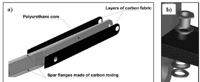
Fig. 7. a) Scheme of composite structures, b) Construction of the labyrinth lock
