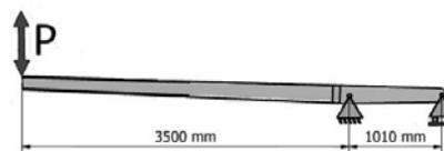
Fig. 1. Scheme of support and loading of spar
