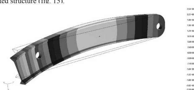
Fig. 13. Spar deflection. Result of FEM analysis. Load  $n=5.7$
