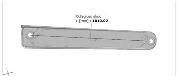
Fig. 20. Spar scan after 10,000 load cycles
