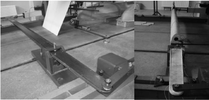
Fig. 3. General view of test stand with attached spar
