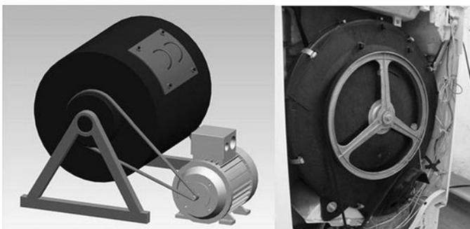
Fig. 1. The concept and implementation of laboratory stand for testing of resistance to abrasion
