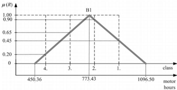
Fig. 10. Reading the coordinates for reliability of bulldozer B1
