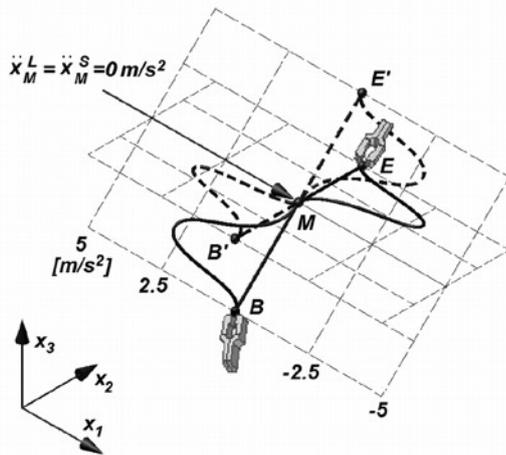
Fig. 4. Resultant acceleration course along planned BME trajectory and ancillary segments
