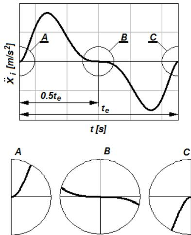
Fig. 1. Acceleration profile described by a 7<sup>th</sup> - degree polynomial
