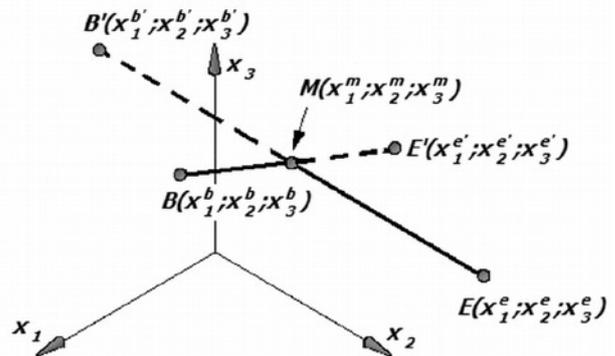
Fig. 2. Planned trajectory  $BME$  and  $ME'$  and  $B'M$  ancillary segments
