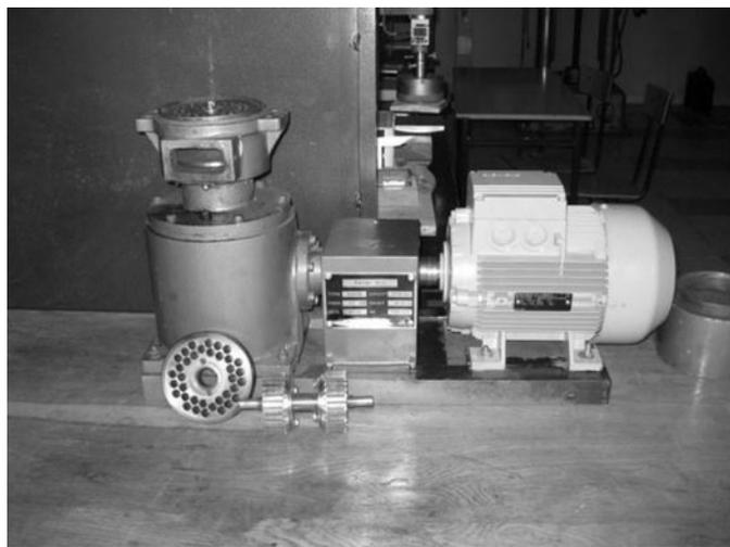
Fig. 3. Laboratory granulator
