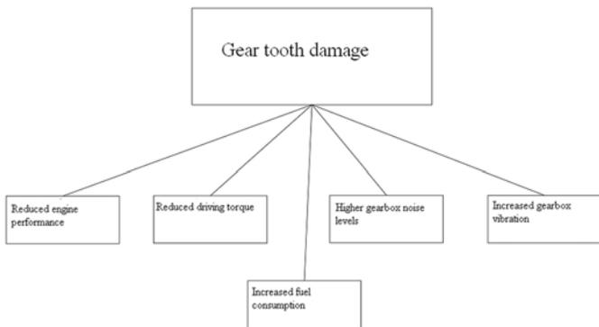
Fig. 6. Diagnostic symptoms of gear tooth damage
