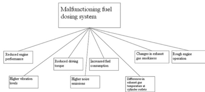
Fig. 11. Diagnostic symptoms of fuel dosing system malfunctions
