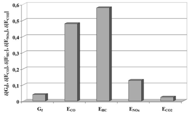
Fig. 6. Relative ranges of the average fuel flow intensity ( $G_f$ ) and of the average intensity of emission of carbon monoxide ( $E_{CO}$ ), hydrocarbons ( $E_{HC}$ ), nitrogen oxides ( $E_{NOx}$ ), and carbon dioxide ( $E_{CO2}$ ) for negative and positive vehicle accelerations in the CT test
