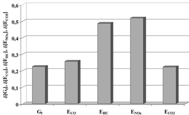
Fig. 13. Average values of the average fuel flow intensity ( $G_f$ ) and of the average intensity of the emission of carbon monoxide ( $E_{CO}$ ), hydrocarbons ( $E_{HC}$ ), nitrogen oxides ( $E_{NOx}$ ), and carbon dioxide ( $E_{CO2}$ ) for negative ( $a < 0$ ) and positive ( $a > 0$ ) vehicle accelerations in the PIMOT tests
