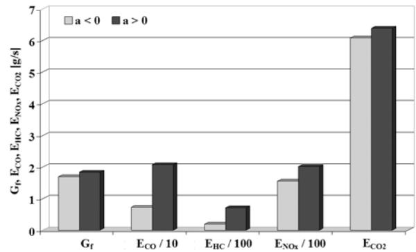
Fig. 5. Average values of the average fuel flow intensity ( $G_f$ ) and of the average intensity of emission of carbon monoxide ( $E_{CO}$ ), hydrocarbons ( $E_{HC}$ ), nitrogen oxides ( $E_{NOx}$ ), and carbon dioxide ( $E_{CO2}$ ) for negative ( $a < 0$ ) and positive ( $a > 0$ ) vehicle accelerations in the CT test
