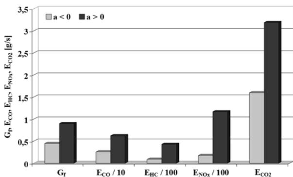
Fig. 14. Relative ranges of the average fuel flow intensity ( $G_f$ ) and of the average intensity of the emission of carbon monoxide ( $E_{CO}$ ), hydrocarbons ( $E_{HC}$ ), nitrogen oxides ( $E_{NOx}$ ), and carbon dioxide ( $E_{CO2}$ ) for negative and positive vehicle accelerations in the PIMOT tests
