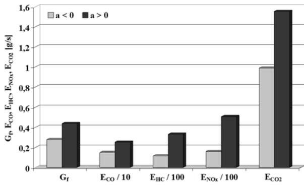
Fig. 12. Relative ranges of the average fuel flow intensity ( $G_f$ ) and of the average intensity of the emission of carbon monoxide ( $E_{CO}$ ), hydrocarbons ( $E_{HC}$ ), nitrogen oxides ( $E_{NOx}$ ), and carbon dioxide ( $E_{CO2}$ ) for negative and positive vehicle accelerations in the HT test
