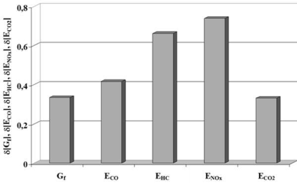
Fig. 7. Average values of the average fuel flow intensity ( $G_f$ ) and of the average intensity of the emission of carbon monoxide ( $E_{CO}$ ), hydrocarbons ( $E_{HC}$ ), nitrogen oxides ( $E_{NOx}$ ), and carbon dioxide ( $E_{CO2}$ ) for negative ( $a < 0$ ) and positive ( $a > 0$ ) vehicle accelerations in the UT test
