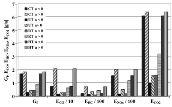
Fig. 10. Relative ranges of the average fuel flow intensity ( $G_f$ ) and of the average intensity of the emission of carbon monoxide ( $E_{CO}$ ), hydrocarbons ( $E_{HC}$ ), nitrogen oxides ( $E_{NOx}$ ), and carbon dioxide ( $E_{CO2}$ ) for negative and positive vehicle accelerations in the RT test
