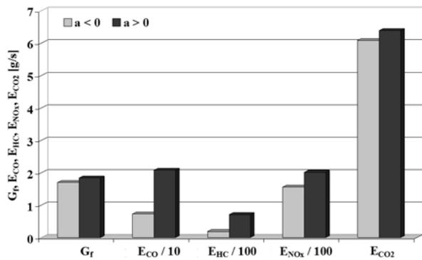
Fig. 8. Relative ranges of the average fuel flow intensity ( $G_f$ ) and of the average intensity of the emission of carbon monoxide ( $E_{CO}$ ), hydrocarbons ( $E_{HC}$ ), nitrogen oxides ( $E_{NOx}$ ), and carbon dioxide ( $E_{CO2}$ ) for negative and positive vehicle accelerations in the UT test
