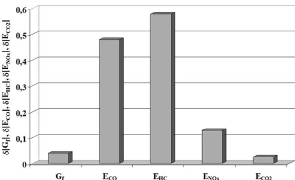
Fig. 9. Average values of the average fuel flow intensity ( $G_f$ ) and of the average intensity of the emission of carbon monoxide ( $E_{CO}$ ), hydrocarbons ( $E_{HC}$ ), nitrogen oxides ( $E_{NOx}$ ), and carbon dioxide ( $E_{CO2}$ ) for negative ( $a < 0$ ) and positive ( $a > 0$ ) vehicle accelerations in the RT test
