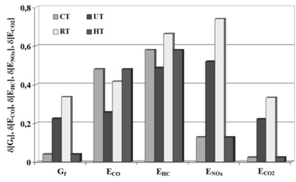
Fig. 11. Average values of the average fuel flow intensity ( $G_f$ ) and of the average intensity of the emission of carbon monoxide ( $E_{CO}$ ), hydrocarbons ( $E_{HC}$ ), nitrogen oxides ( $E_{NOx}$ ), and carbon dioxide ( $E_{CO2}$ ) for negative ( $a < 0$ ) and positive ( $a > 0$ ) vehicle accelerations in the HT test
