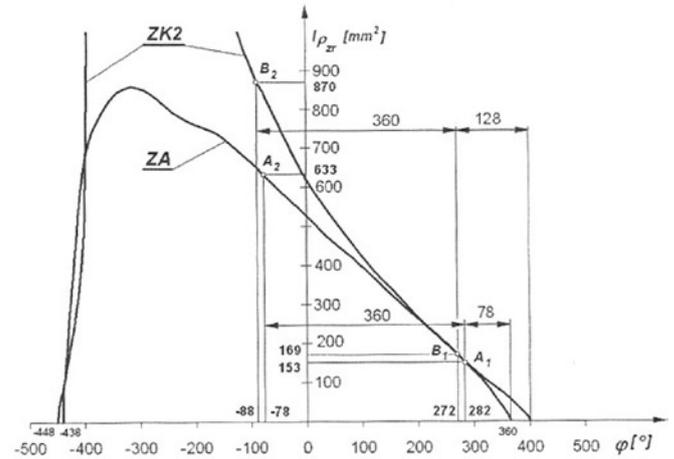
Fig. 7. The dependency of contact line length and curvature radius from worm screw rotation
