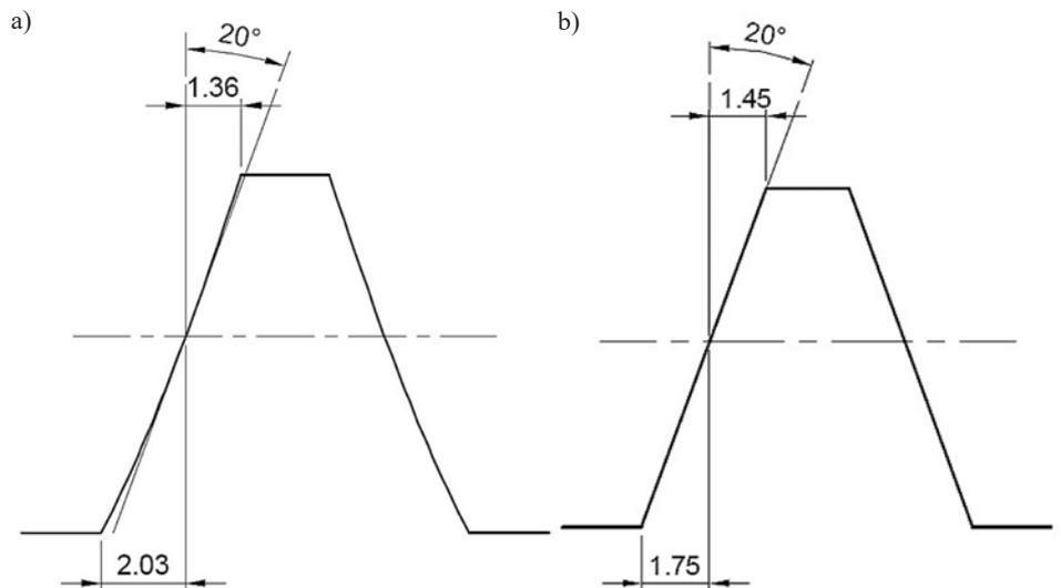
Fig. 3. Axial tooth profile: a) concave b) linear
