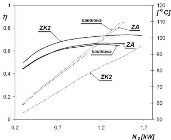
Fig. 6. Gearbox efficiency as a function of load
