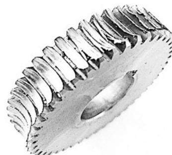
Fig. 1. Wormwheel tooth damage resulting from excessive loads.
