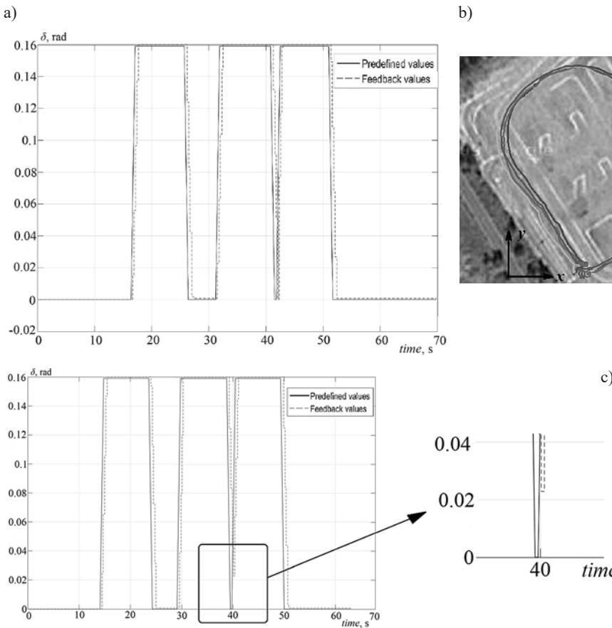
*Fig. 5. Data of the performed experimental drives while using Eq. (17): a – the predefined values and the experimental drive feedback data values of the actual steering angle of the front wheels; b – example of the performed experimental drives while moving in a path, re-planned while using Eq. (17); c – the experimental drive feedback data values of the actual steering angle of the front wheels when front wheels were not returned to neutral position*
