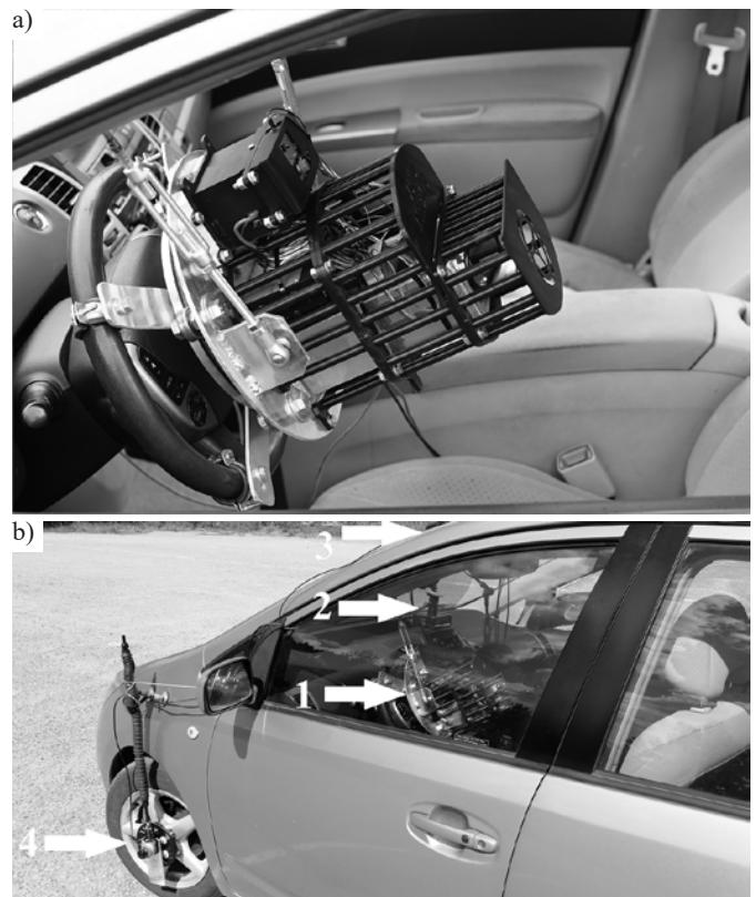
Fig. 2. Experimental research: a – automated steering device mounted on the test vehicle; b – autonomous test vehicle with 1 – automated steering device, 2 – GPS tracker, 3 – GPS antenna, 4 – angular velocity sensor
