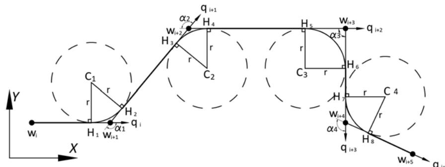
Fig. 1. Scheme of path re-planning using the vector based Dubins path approach
