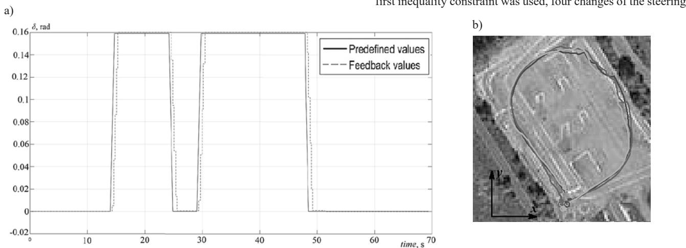
Fig. 4. Data of the performed experimental drives while using Eq. (14): a – the predefined values and the experimental drive feedback data values of the actual steering angle of the front wheels; b – example of the performed experimental drives while moving in a path, re-planned while using Eq. (14)
