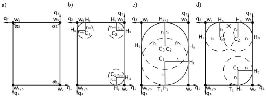
Fig. 3. Basic schemes of the predefined and re-planned paths: a – the predefined path; b – the path re-planned while using the non-modified Dubins path approach; c – the path re-planned while using Eq. (14); d – the path re-planned while using Eq. (17)
