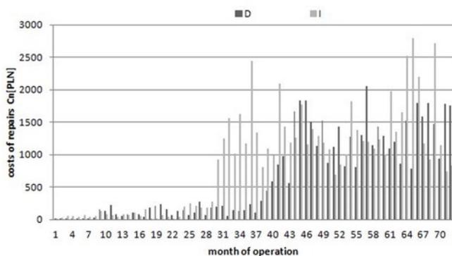
Fig. 3. Monthly costs of repairs per 1 bus [9]
