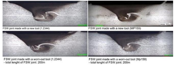
Fig. 9. Cross-section of the FSW joints welded using new and worn tools
