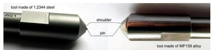
Fig. 1. FSW tools used in wear testing
