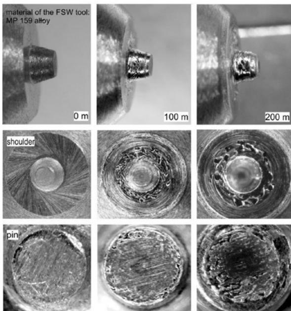
Fig. 8. Visual inspection of the working surface of the FSW tool made of MP159 alloy following individual stages of wear tests
