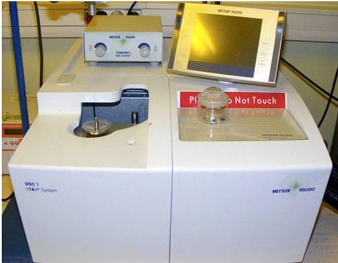
Fig. 1. Differential scanning calorimeter Mettler Toledo DSC 1
