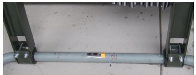
Fig. 5. Stabilizer with glued-on strain gauge
